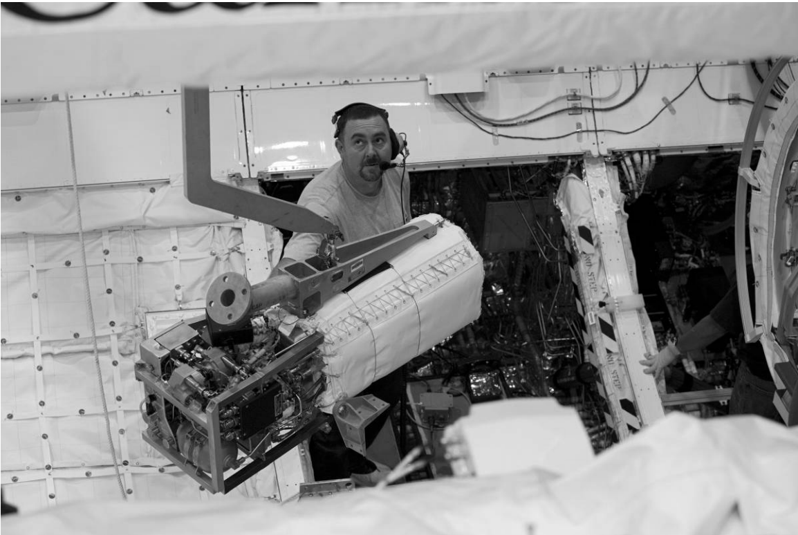
Figure No. A-25. One of Discovery 's fuel cells being reinstalled following drain and purge operations conducted as part of the shuttle transition and retirement efforts, December 9, 2011. Source: NASA Kennedy Space Center, KSC-2011-8202, accessed May 2012, at http://mediaarchive.ksc.nasa.gov .
