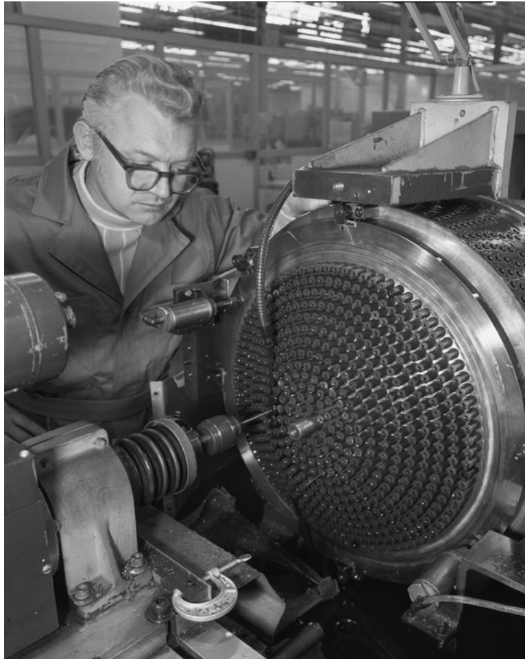
Figure C-25. A technician reams holes into the SSME main injector body at Rocketdyne's Canoga Park, California, facility, direction unknown, August 1, 1978. Source: George C. Marshall Space Flight Center, Marshall Image Exchange (MIX), 7779474, accessed at http://mix.msfc.nasa.gov/ .
