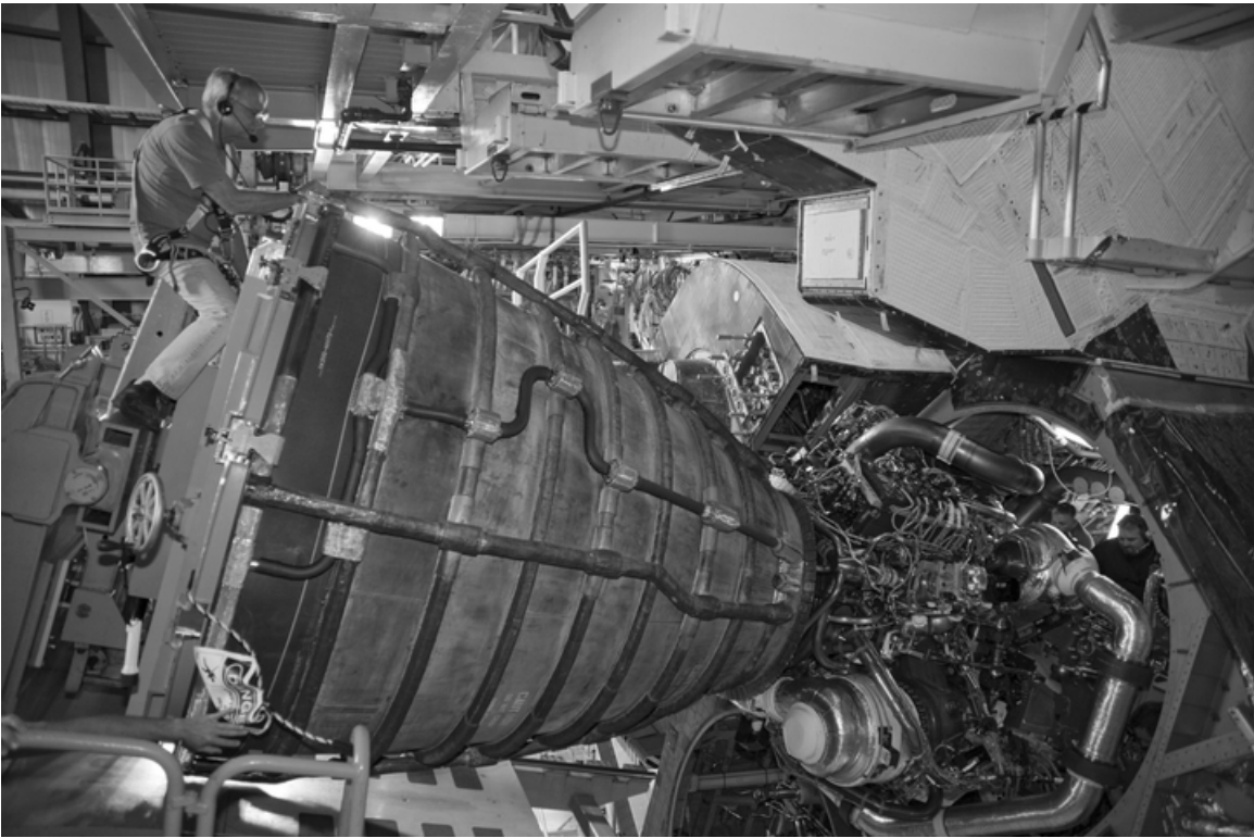
Figure C-42. A SSME being maneuvered into engine position No. 1 of Discovery , OPF-3, camera facing west, June 30, 2010.
