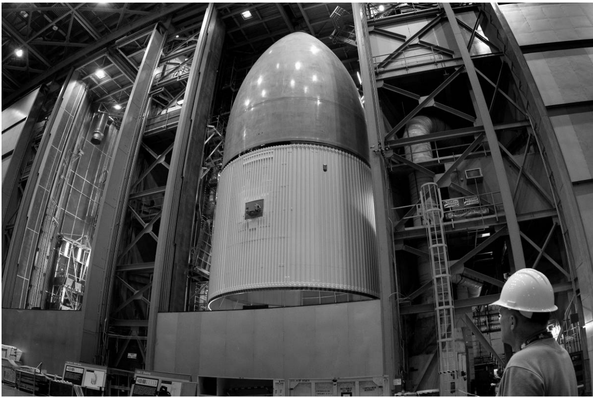
Figure D-33. LO2/intertank combination for ET-138 in Cell H at MAF, November 12, 2009. Source: NASA, Johnson Space Center, Imagery Online, jsc2010e009722.
