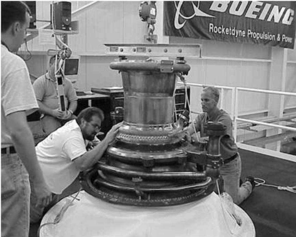
Figure C-31. Technicians attach the Main Combustion Chamber to the Nozzle in the SSMEPF at Kennedy Space Center, camera facing northeast, date unknown. Source: George C. Marshall Space Flight Center.
