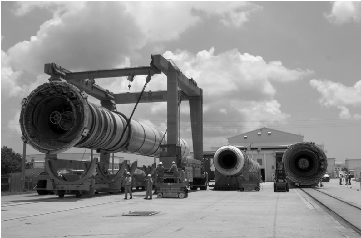
Figure No. E-35. Crane lifts SRB used during Atlantis ' STS-132 launch onto a tracked dolly at Hangar AF Disassembly Facility, May 18, 2010.
