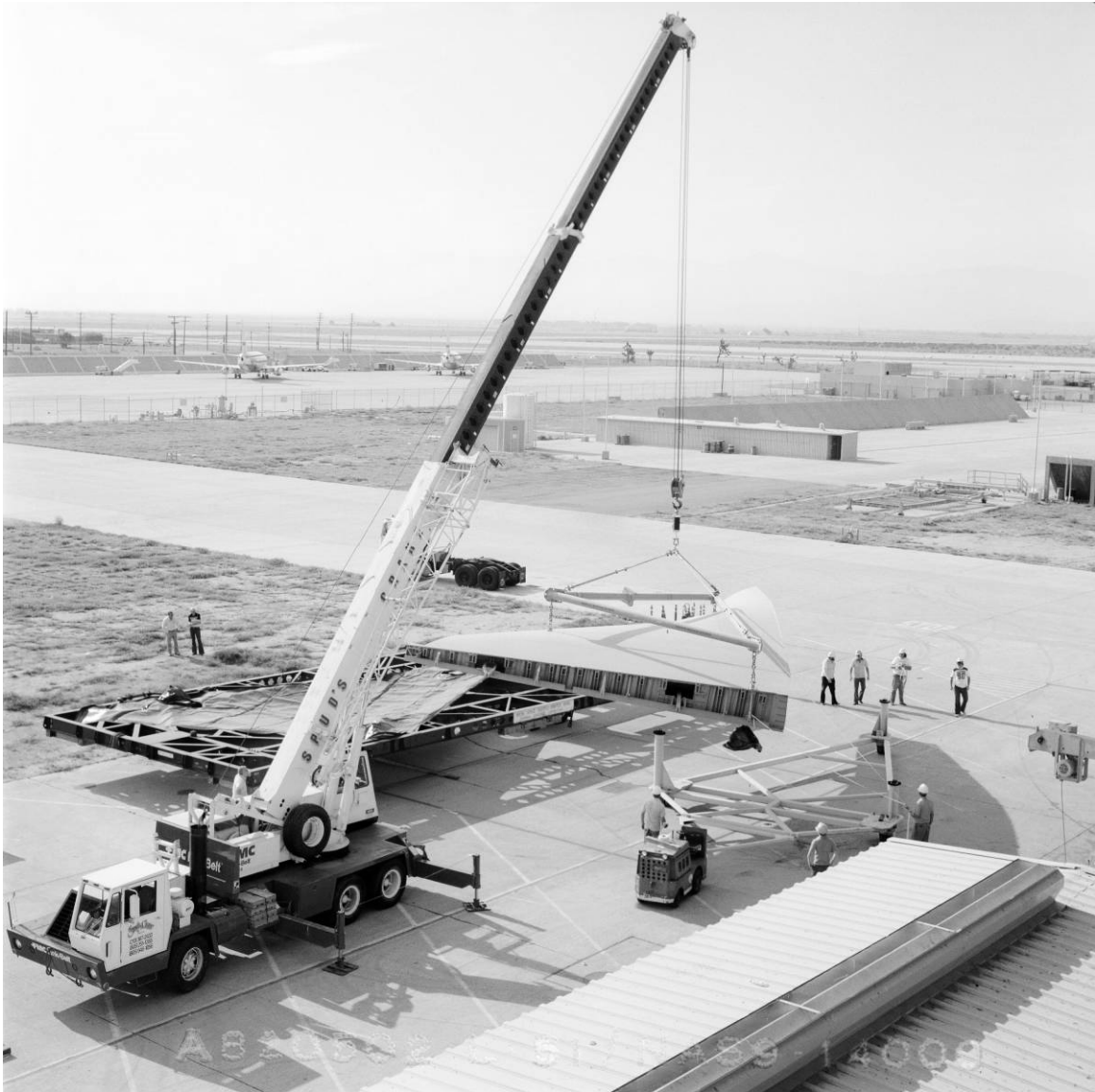
Figure B-22. Discovery's port wing being offloaded from transporter at AFP 42, May 2, 1982. Source: NASA, Johnson Space Center Image Repository, JSC2010-03283.
