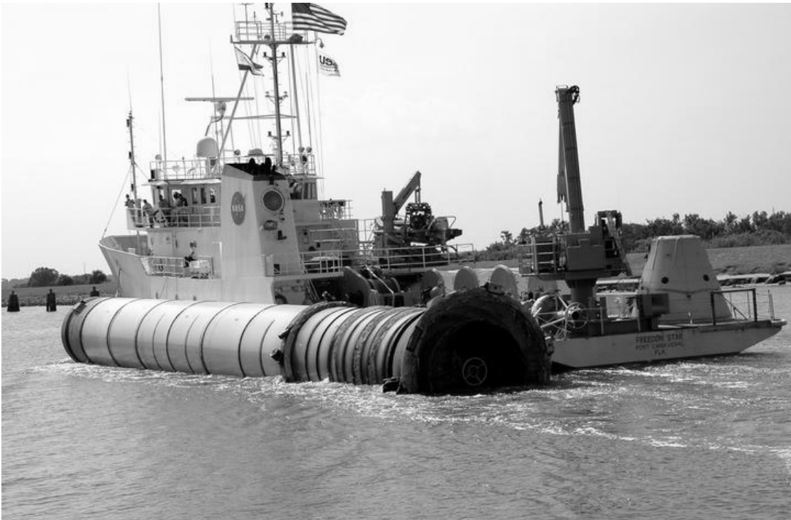
Figure No. E-33. SRB retrieval ship, Freedom Star , towing spent SRB from the STS-114 launch, July 27, 2005.
