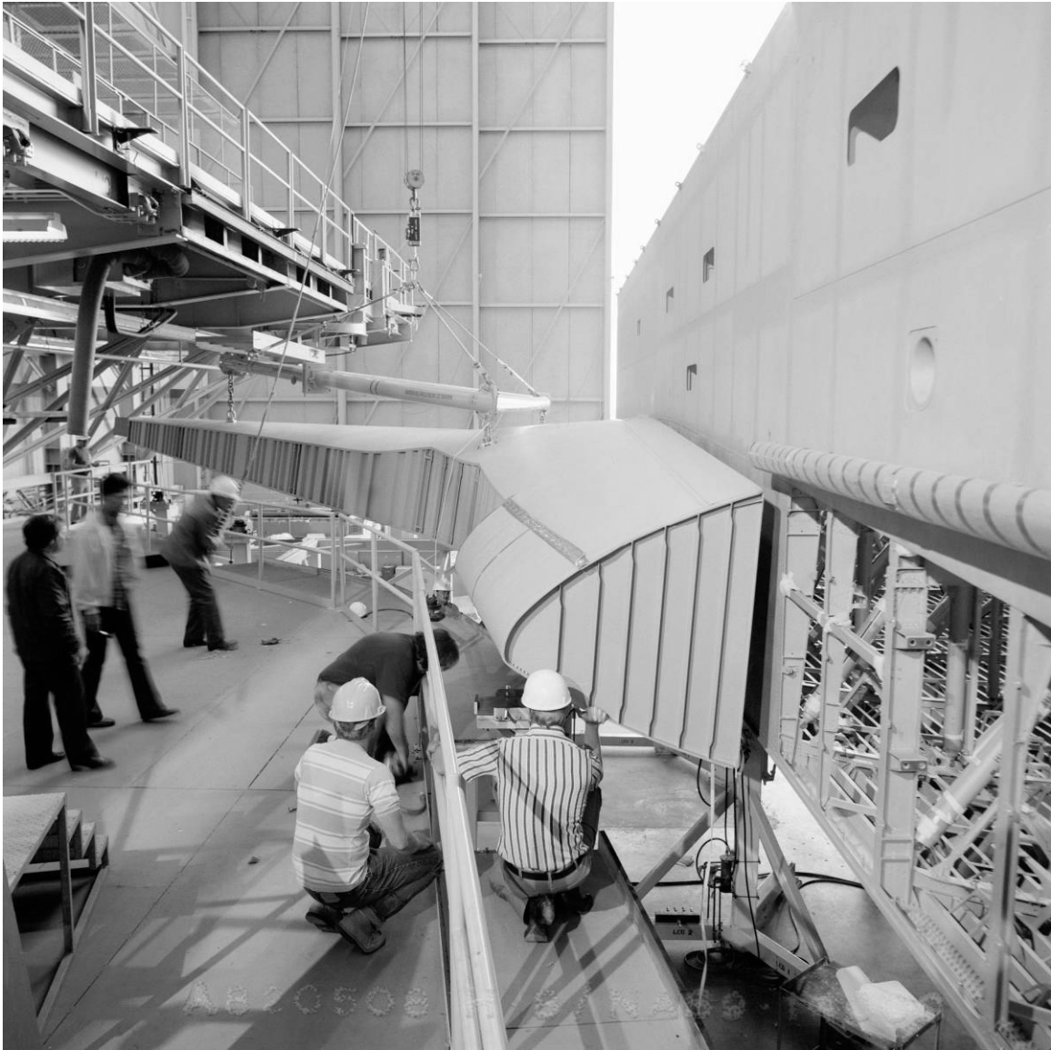
Figure B-23. Discovery's starboard wing being attached to the midfuselage in High Bay 2, AFP 42, May 8, 1982.
