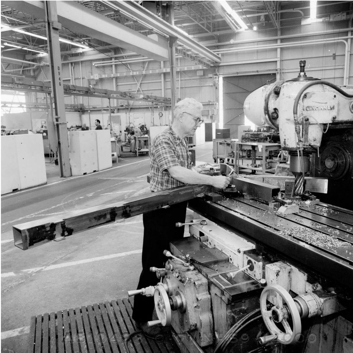
Figure B-15. Manufacturing of a vertical truss for the thrust structure of Discovery's aft fuselage, NAR Building 1, Downey, California, April 23, 1981. Source: NASA, Johnson Space Center Image Repository, JSC2010-03093.
