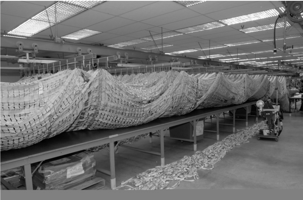
Figure No. E-44. Parachute from Endeavour's STS-126 mission is suspended from a hanging monorail system at the KSC Parachute Refurbishment Facility, November 19, 2008.
