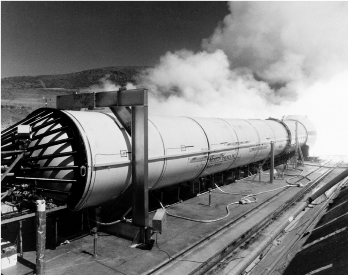
Figure No. E-3. Test firing of Development Motor-8 (DM-8) in test stand at Morton Thiokol's Wasatch, Utah, facility, August 27, 1987.
