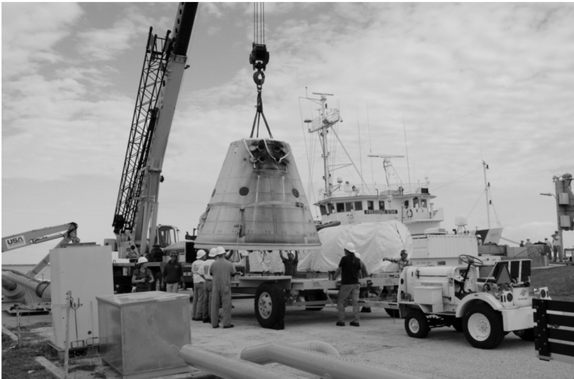
Figure No. E-36. The frustum of a SRB used during Discovery's launch on mission STS-119 is lifted onto a transporter at the Hangar AF dock, March 18, 2009. Source: NASA Kennedy Space Center, KSC-2009-2140, accessed at http://mediaarchive.ksc.nasa.gov .
