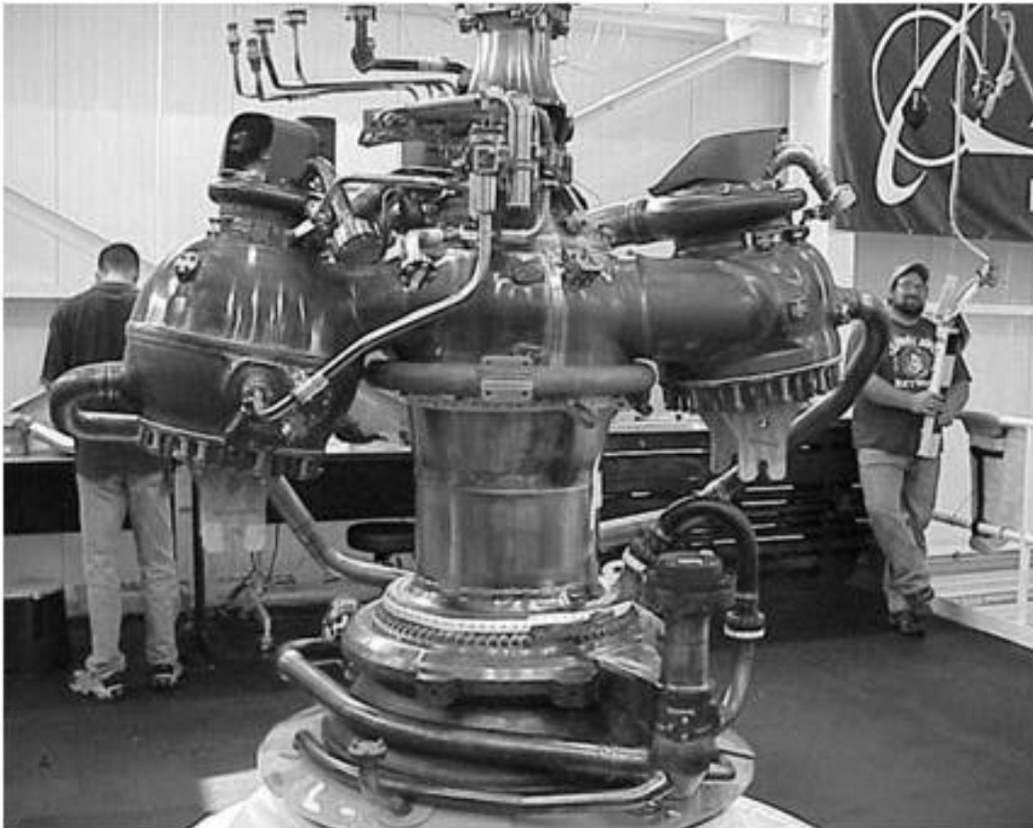
Figure C-32. Attachment of the Powerhead to the Main Combustion Chamber, SSMEPF, camera facing northeast, date unknown.
