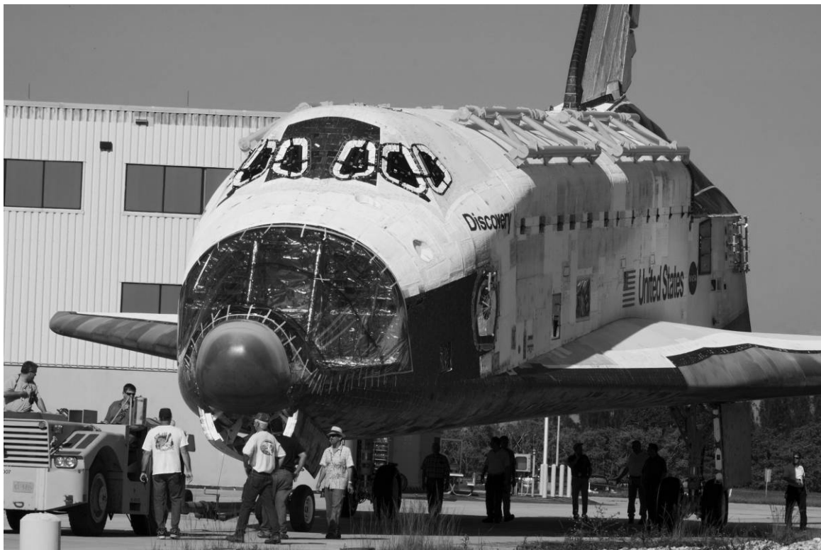
Figure No. A-22. View of Discovery without her FRCS module and OMS pods, which were sent to the White Sands Test Facility in New Mexico for deservicing and cleaning as part of the shuttle transition and retirement efforts, July 13, 2011.
