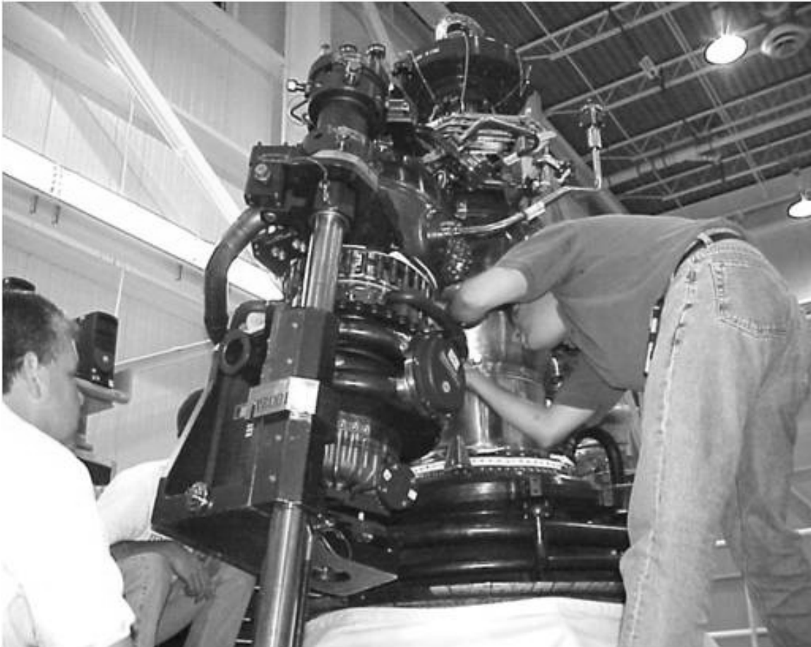
Figure C-33. A technician attaches the High Pressure Oxidizer Turbopump to the SSME, SSMEPF, camera facing northeast, date unknown. Source: George C. Marshall Space Flight Center.
