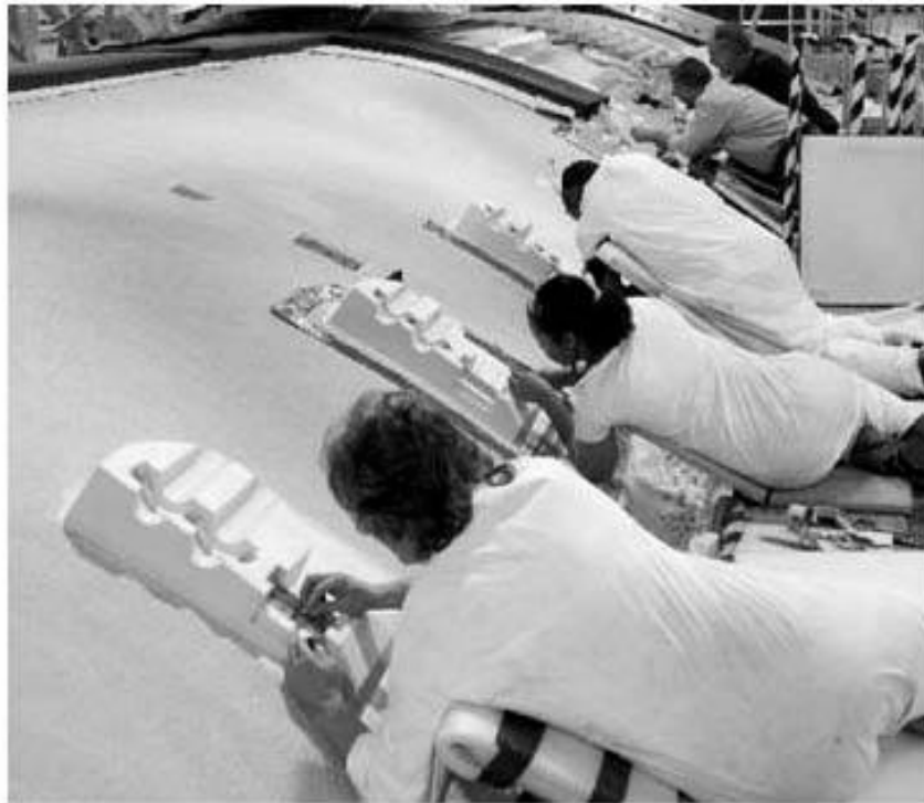
Figure D-12. Lockheed Martin technicians installing ice/frost ramps. Source: NASA, NASA Facts: Space Shuttle External Tank ET-128, STS-124 , 2; accessed at http://www.nasa.gov/centers/marshall/pdf/228641main_8-368946_%282%29.pdf .
