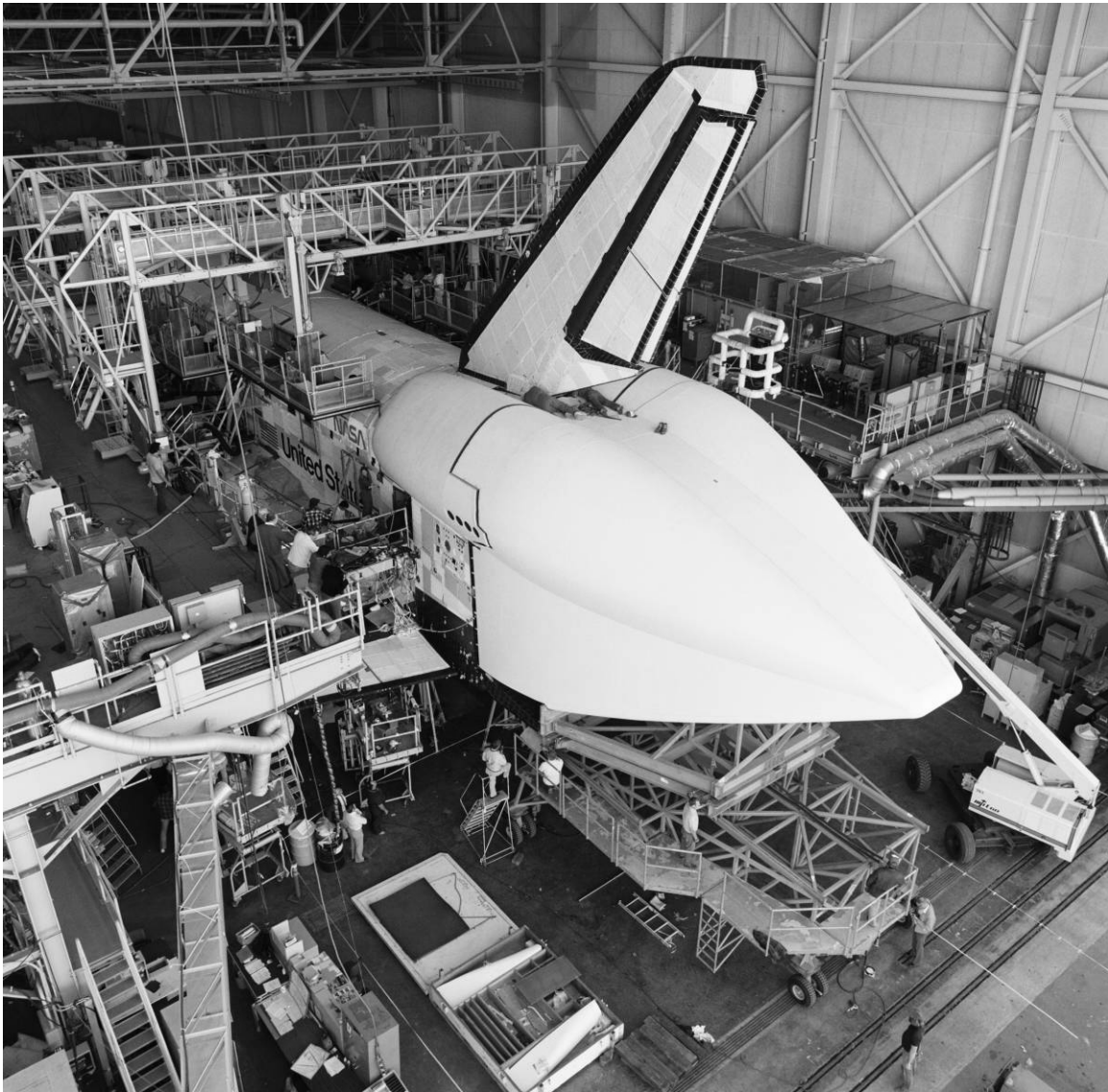
Figure B-58. Installation of tail cone onto Discovery for transport to DFRC, High Bay 2, AFP 42, October 10, 1983.
